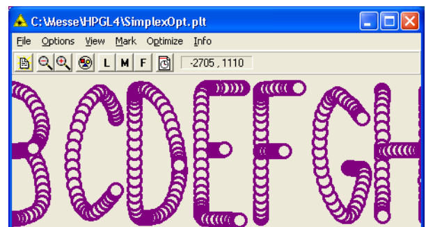
Figure 6: Simulation with the same laser parameters as in Figure 5, but now 1300 characters per second with a marking speed 4.5 m/s.
