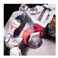
Laser processing systems use galvanometer scanners as highly dynamic drives to precisely position the laser onto a workpiece. Mirrors mounted on the galvos allow the laser beam to be precisely positioned for the particular application. Core components are a galvo motor (based on moving magnets) and a position detector. Until now, digital position detectors sensed a scale coded on a disc which is bonded to the scanner rotor. But this
