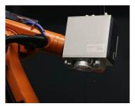
Remote welding – with scan heads mounted on industrial robots – is widespread in auto manufacturing, and offers considerable potential for other branches, too. Here, the scan system manages laser fine-positioning, thus eliminating time-robbing robot repositioning. This has significantly boosted beam utilization rates and manufacturing productivity over the past few years.
